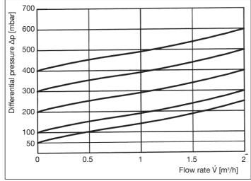
Flow chart bypass (pressure relief device)
