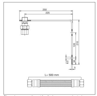
Dimensions connection set for diaphragm expansion tanks
