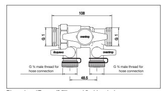
Dimensions "Regusol" filling and flushing device
