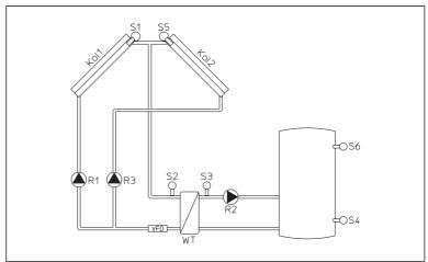
For 2 collector fields with storage cylinder connection for simple operation
