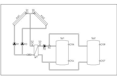
For 2 collector fields with storage cylinder connection for loading of 2 separate storage cylinders
