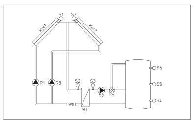
For 2 collector fields with storage cylinder connection for loading section by section
