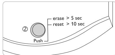
The operating control LED ② indicates the operating status of the Datalog CS-BS-1 by issuing flashing signals and colours.
