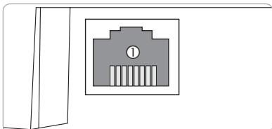
The integrated LAN connector ① is located on the right-hand side of the device. The LAN connector supports transfer rates of up to 100 MBit per second.
