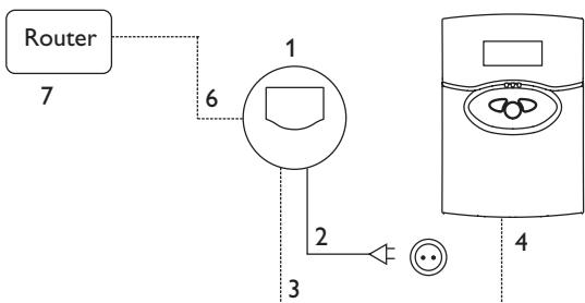
Power supply is carried out via an external mains adapter (terminals 1 and 2). The supply voltage of the mains adapter must be 100 ... 240V~ (50 ... 60 Hz).
