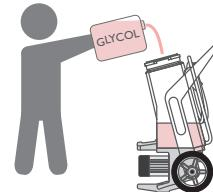
→ Make sure the tank is filled at least to the MIN marking.
