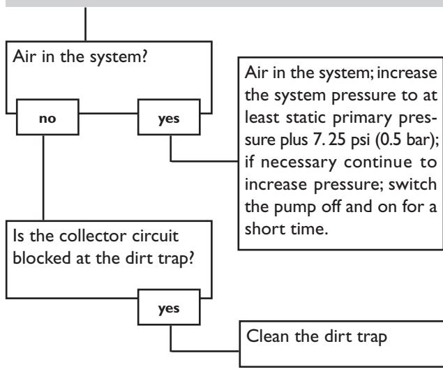
Pump starts for a short moment, switches off, switches on again, etc.
