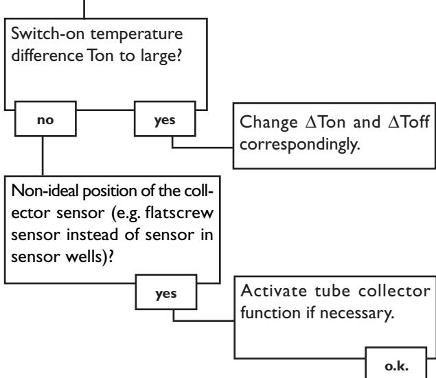
The temperature difference between store and collector increases enormously during operation; the collector circuit cannot dissipate the heat.
