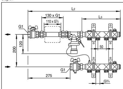
**Illustr. 5:** Heat meter connection set no. 1, straight pattern and stainless steel distributor/collector "Multidis SH" for radiator connection, installation lengths
