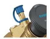
Every HydroCom A is equipped with a HydroPort auxiliary valve as standard. The HydroPort allows snap on connection of accessories. The HydroPort is opened by turning anticlockwise. A quarter turn is sufficient to measure the pressure, a full turn is sufficient to drain and fill.
