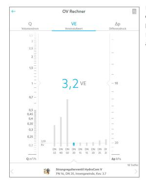
HydroSet is the digital slide ruler for Oventrop regulating valves. HydroSet calculates the Kv value after input of desired flow and available differential pressure. Further the presetting position of the selected valve.
