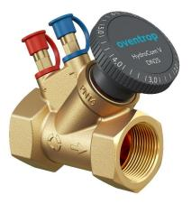
The HydroCom V is a double regulating valve with variable orifice for the static hydronic balancing of pipelines in closed heating and cooling systems.
