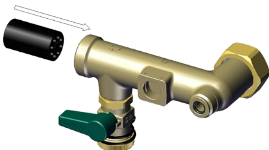
Fig. 35: Installation of the measuring turbine
