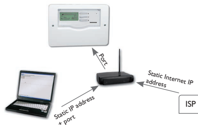
Schematic representation: Remote access to the Datalog CS-BS-6, router with static Internet IP address.
