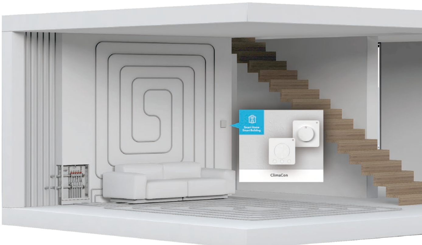
Fig. 1: Installation scheme (example)
