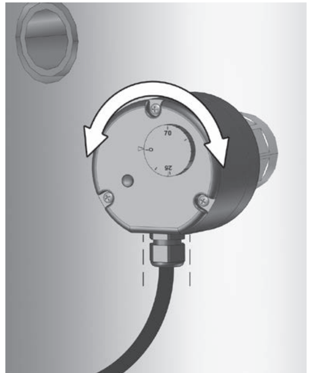
Illustration 13: Align screwed cable gland
