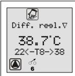
Display of the temperature of the energy sink sensor in the "Information" menu, with minimum and maximum values. The corresponding measuring point – here T8 – is also displayed.
