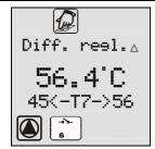
Display of the temperature of the energy source sensor in the "Information" menu, with minimum and maximum values. The corresponding measuring point – here T7 – is also displayed.
