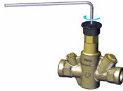
Fig. 6: Setting the temperature setpoint
