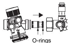
4. Mount seal and tighten collar nut
