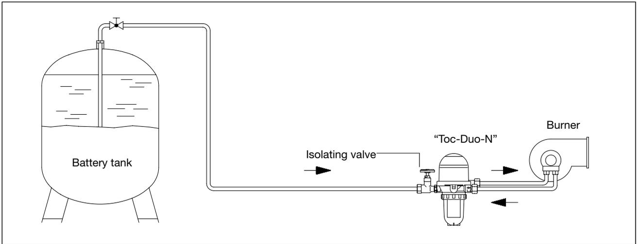
Installation of the "Toc-Duo-N" above the oil level, e.g. underground tank
