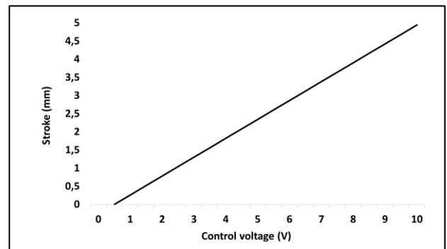
Stroke-control voltage-characteristic line (max. stroke without valve)
