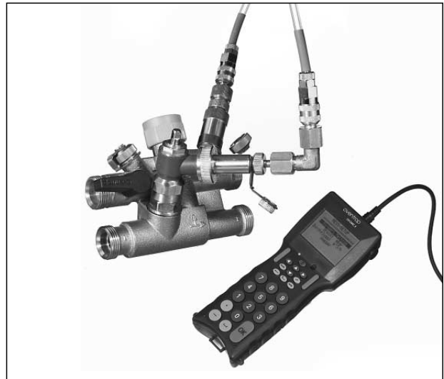
Illustr. 6 Differential pressure measurement of terminal unit
