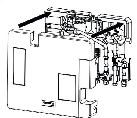
*Abb. 2: Installation of the thermal insulation cover*
