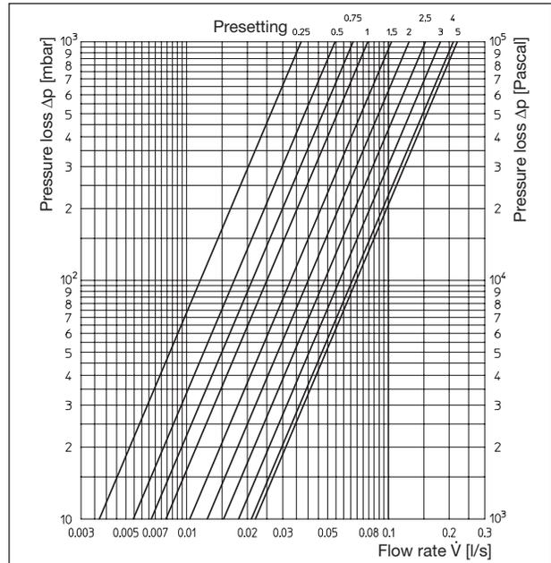
Regulating insert, 2 K P-deviation, bypass presetting 1.9 (50%)
