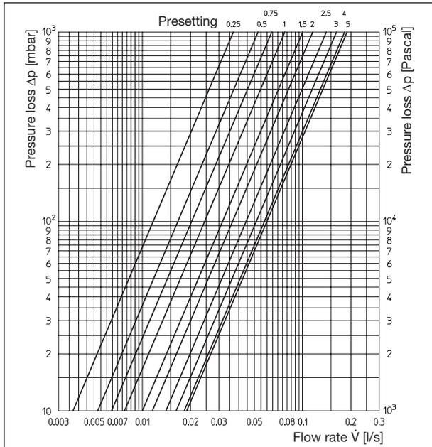
Regulating insert, 2 K P-deviation, bypass presetting 1.4 (25%)
