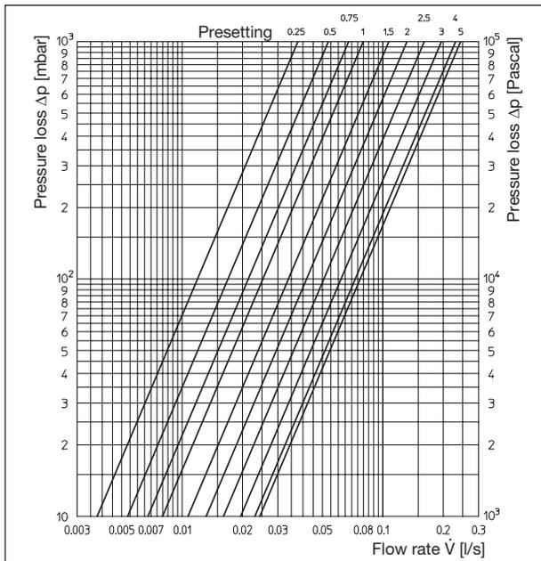
Regulating insert, 2 K P-deviation, bypass presetting 2.3 (75%)
