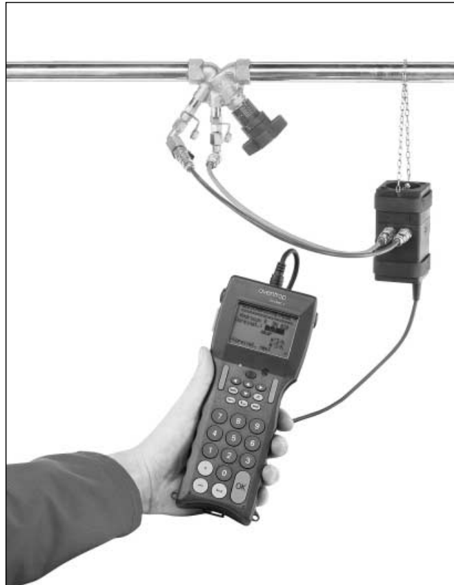
“OV-DMC 2” item no. 106 91 77 with double regulating and commissioning valve “Hydrocontrol R”
