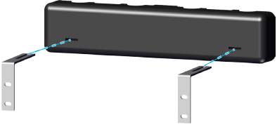
Fig. 4: Position of the wall brackets
