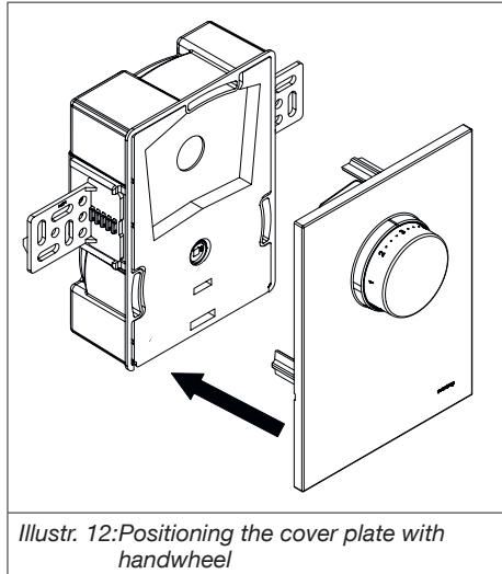
*Illustr. 12:Positioning the cover plate with handwheel*
