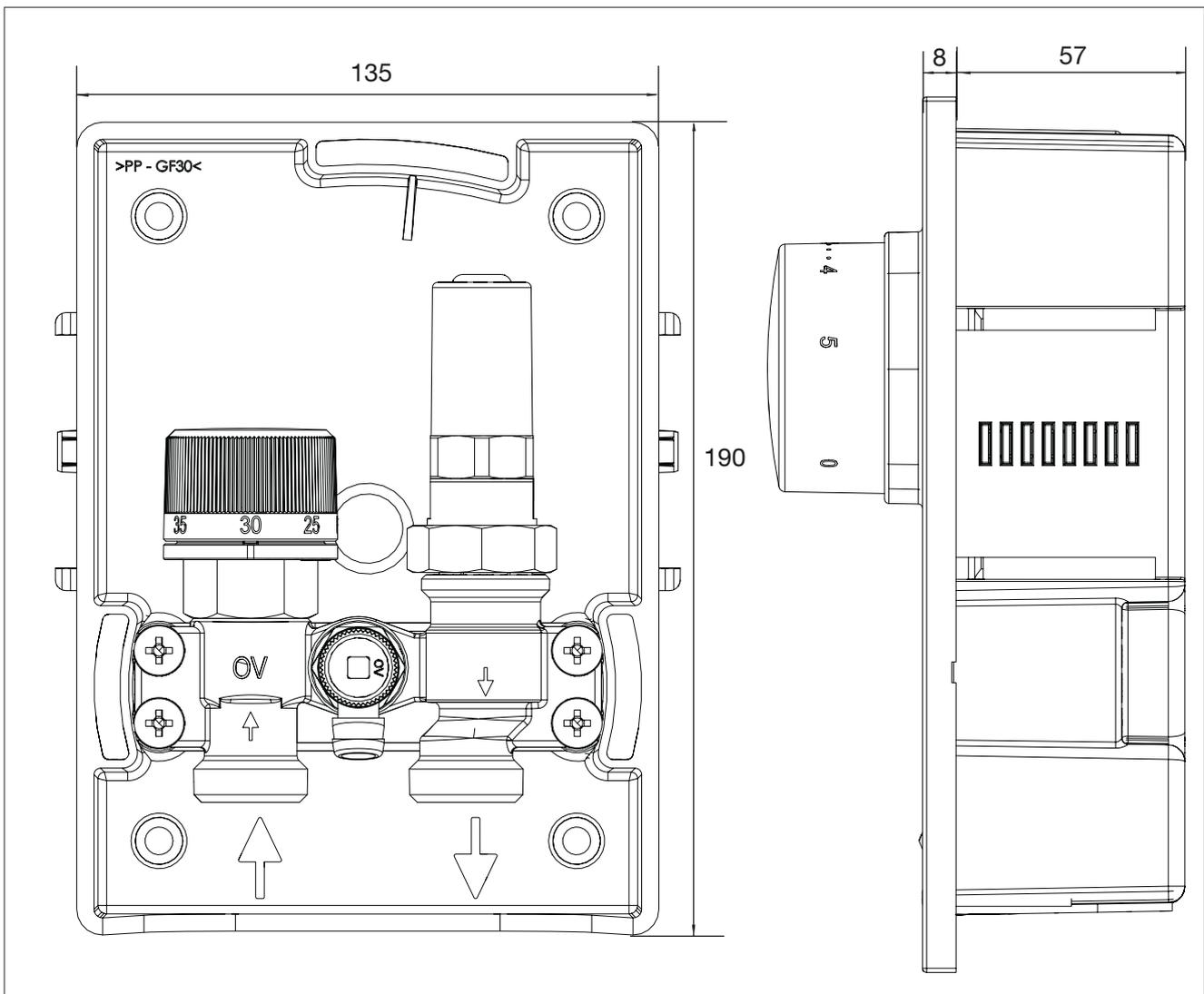
Illust. 2: Dimensions “Unibox T-RTL” in mm (front and side view)
