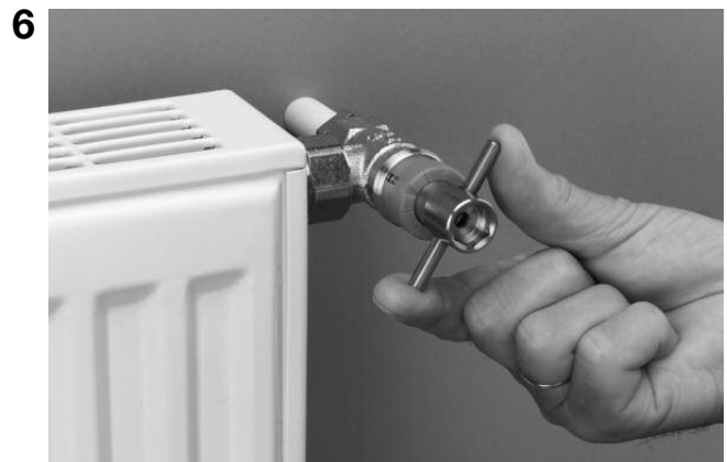
6 Presetting is carried out by turning anticlockwise (one complete turn corresponds to presetting 1 etc., max. of 6 turns).
