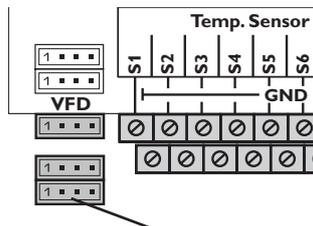
Conectar el sensor **digital Grundfos Direct Sensor™ VFD 2-40 I Fast** a la entrada VFD.
