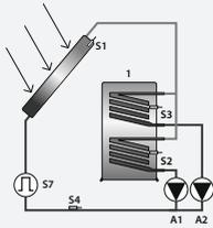
**6.3 Diagram 2: 1 collector, 2 storage tanks with 2 pumps**
