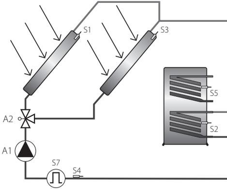
**i** Type 3: two collectors, one storage tank with a three-way valve:
