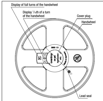
Illustr. 7 Locking the handwheel DN 200 - DN 300
