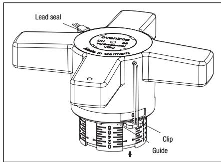
Illustr. 6 Locking the handwheel DN 65 - DN 150
