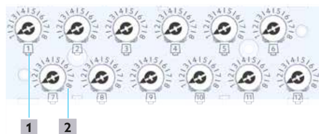
Fig. 6: Control zone assignment F 300
