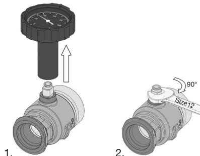
Illust. 21: Isolation of the pump ball valves
