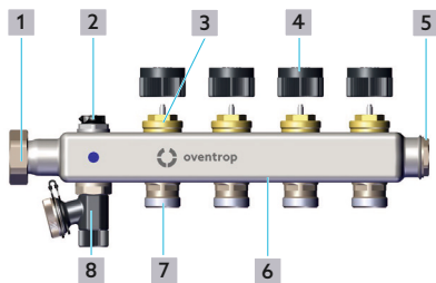
Fig. 2: Design of the return collector
