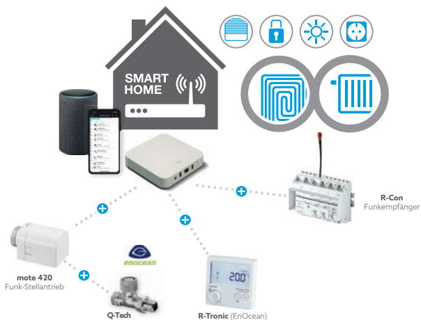
Illust. 1: Automatic presetting and balancing with the wibutler pro gateway and Q-Tech technology
