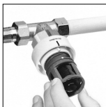
Photo 13: Remove handgrip. Turn sensor casing to the right until it is fully screwed into the body of the thermostat, then turn to the left again until the calibration mark (bore or white stroke) is in line with the indicator mark.
