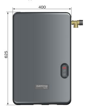
Fig. 5: Dimensions Regumaq X-25 with upper shell
