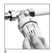
Photo 6: Replace the handgrip so that figure "3" is in line with the indicator mark.
