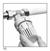
Photo 11: The handgrip now is to be replaced so that figure "2" is in line with the indicator mark. The setting is now blocked in position "2" (approx. 16 °C). Push down handgrip with hand firmly to secure.
