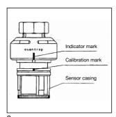
Photo 2: After having removed the handgrip: Turn the sensor casing to the left until the calibration mark (bore or white stroke) is in line with the indicator mark.
