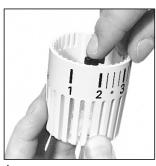
Photo 4: To limit the minimum control range, e.g. at figure "2" (equals approx. 16 °C), one clip should be fitted into the groove immediately **before** figure "2" as illustrated.
