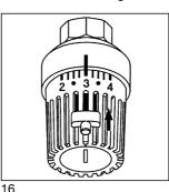
Illustr.16: Blocked temperature setting: Insert tool (item no. 1989100) on top of the handgrip so that one bridge is in the groove immediately before and one bridge in the groove immediately after the indicator mark. Push tool in direction of arrow to loosen the clips. Remove tool.
