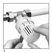
Photo 1: Remove the handgrip with the tool (item no. 1989100) or with a pin, e.g. with the push button of a pen. Insert the tool/pin in the hole provided on the lower side of the thermostat. By turning the handgrip to the shut-off position, it is easily removed (compare photo 16).
