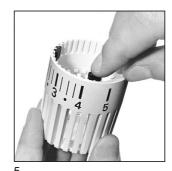
Photo 5: To limit the maximum control range, e.g. at figure "4" (equals approx. 24°C), the second clip should be fitted into the groove immediately **after** figure "4". (The groove directly opposite figure "4" thus remains free.).
