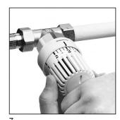
Photo 7: Push down handgrip with hand to secure. The control range of the thermostat is now limited and you can only set values between figure "2" and "4" (approx. 16 °C – 24 °C).
