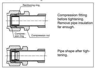
When using thin walled and very soft pipes, reinforcing sleeves have to be used. The reinforcing sleeve supports the pipe and provides the strength to enable the necessary compression. Reinforcing sleeves cannot be used on pipe with welded seams. The recommendations of the pipe manufacturers have to be observed in any case. If necessary, a practical "test" has to be carried out.
