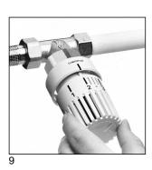
Photo 9: Turn handgrip to figure "2" while pressing it gently. Remove handgrip. (The calibration on the sensor casing is now turned to the right.)
