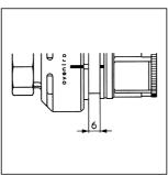
Photo 14: If the sensor casing is for some reason unscrewed completely from the body of the thermostat, please note that when replacing the element, because of the double start thread, the correct start thread is used. After recalibration, the distance between the body and the sensor casing has to be approx. 6 mm.
