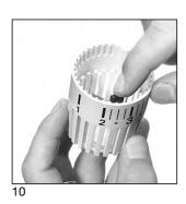
Photo 10: The two clips on the inner side of the handgrip are to be removed as described beside photo 3 and to be placed in the grooves immediately before and after figure "2". (The groove directly opposite figure "2" thus remains free.)
