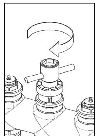
4. Set the arrow of the graduated collar so that it is in line with the marking of the prey setting key.
