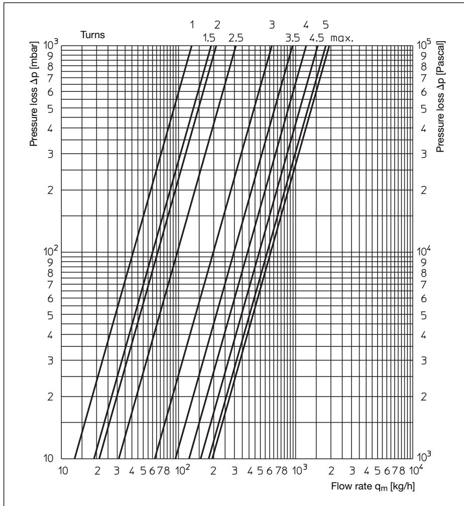
Chart 1: Pressure loss chart regulating insert, valve opened
