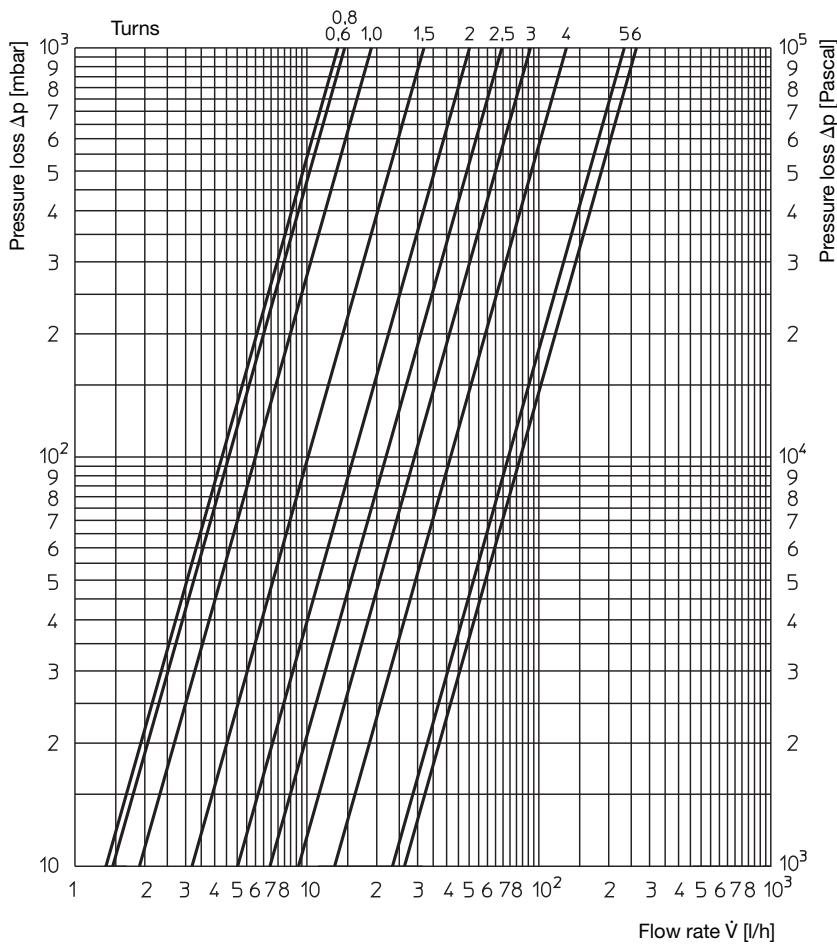
**Chart 2: Pressure loss chart bypass, valve closed**
