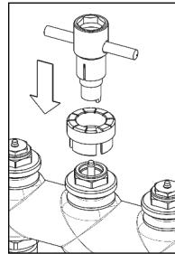
3. Close the bypass by turning the bypass stem clockwise.
